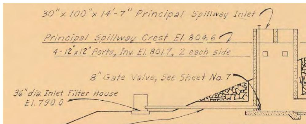
\*Typical intake as originally built. All have been modified with additional trash cages.
